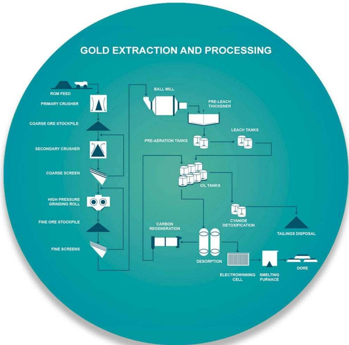
Figure 4 - Mining Production Process (Minerals Council of Australia, 2014)
